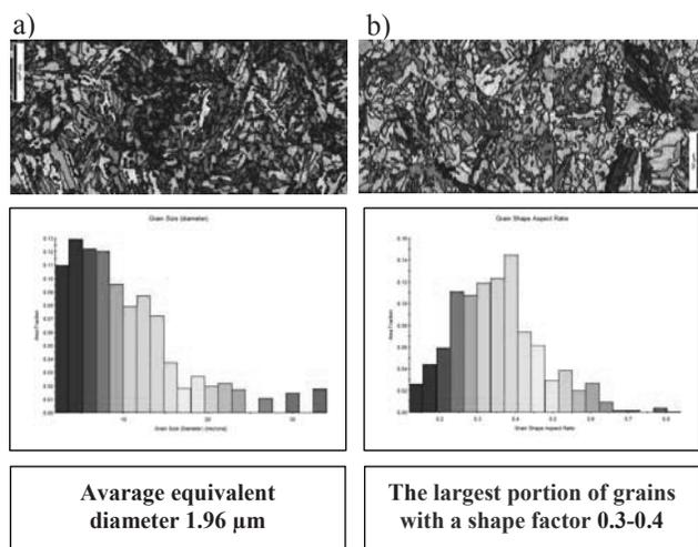
Fig. 8. Characteristic parameters of the microstructure of lower bainite with martensite of tube material made of 7CrMoVTiB10-10 steel for making the membrane walls of the evaporator collector for the boiler with supercritical working parameters disclosed in SEM by the use of EBSD technique: a) the distribution of an average equivalent grain diameter; b) the distribution of grain shape
