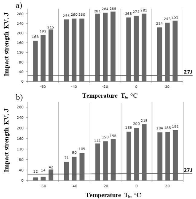
Fig. 12. Impact energy depending on the temperature of tubes material made of 7CrMoVTiB10-10 steel at the room temperature with various forms of bainite and martensite portion: a) Denotation 1; Structure of granular bainite with bainite (66%/34 %), b) Denotation 4, Structure of lower bainite with martensite (65%/35%)
