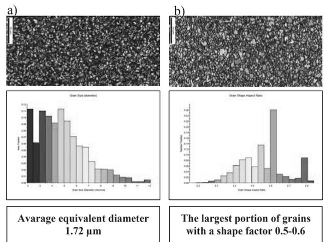
Fig. 6. Characteristic parameters of microstructure of the granular bainite and bainite of tube material made of 7CrMoVTiB10-10 steel for making the membrane walls of the evaporator collector for the boiler with supercritical working parameters disclosed in SEM by EBSD technique: a) the distribution of an average equivalent grain diameter; b) the distribution of grain shape
