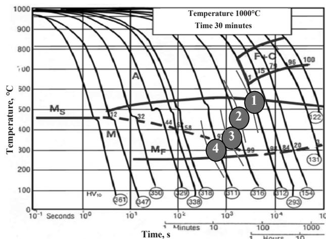
Fig. 4. The estimated cooling rate after austenitising tubes made of 7CrMoVTiB10-10 steel against the background of continuous cooling transformation diagram (TTT<sub>c</sub>) with geometric dimensions: 1)  $\phi$  42.4x7,1 mm, 2)  $\phi$  33.7x5.0 mm, 3)  $\phi$  42.4x7.1 mm, 4)  $\phi$  33.7x5.0 mm
