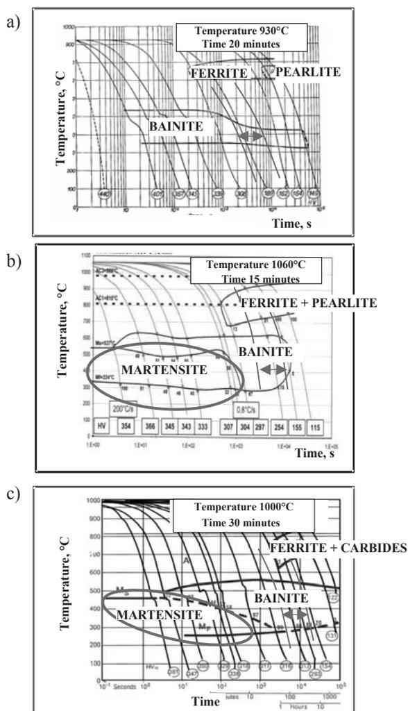
Fig. 2. Comparison of supercooled austenite continuous cooling transformation diagram of ( $TTT_c$ ) of selected low-alloy bainitic steels for power engineering: a) 10CrMo9-10, b) 7CrWVNb9-6, c) 7CrMoVTiB10-10
