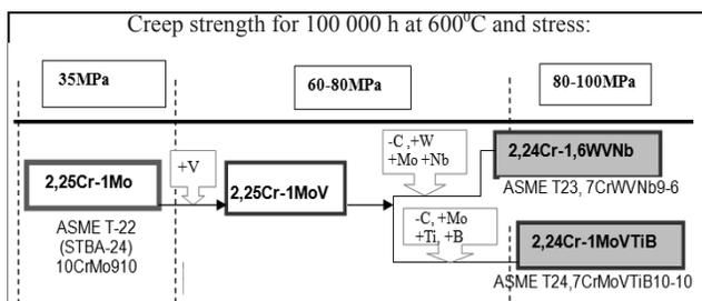
Fig. 1. Development of low-alloy bainitic chromium-molybdenum steel to work in creep conditions [1]
