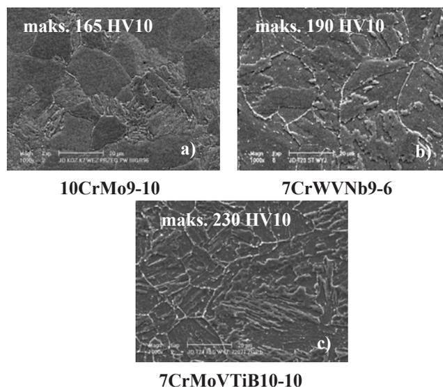
Fig. 3. Comparison of microstructures of selected low-alloy bainitic steels for power engineering, the most commonly appearing in practice: a) 10CrMo9-10, b) 7CrWVNb9-6, c) 7CrMoVTiB10-10 (microstructure observed in a scanning electron microscope)
