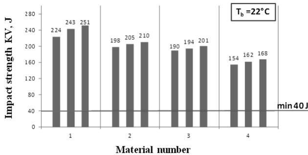
Fig. 11. Impact energy of tubes made of 7CrMoVTiB10-10 steel at the room temperature for gas-tight water wall elements of materials with various forms of bainite and martensite portion Denotation 1; Structure of granular bainite with bainite (66%/34%), Denotation 2, Mixed structure of granular bainite with bainite (63%/37%), Denotation 3; Structure of bainite with ferrite (100%/bainite), Denotation 4, Structure of lower bainite with martensite (65%/35%)
